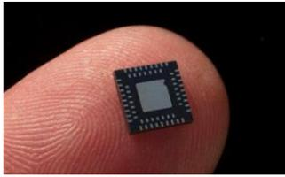
link transistors together, the interaction of which allows computers to make very simple computational decisions. All of this is engineered on a small flat piece - literally a “chip” - of semiconductor material. **Billions** of tiny transistors are integrated on this digital circuit, itself the size of a baby’s fingernail. They make computing power simply explosive.
