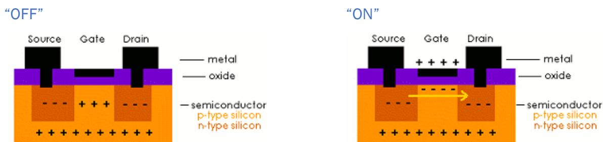
When applying a small positive current to the p-type silicon, the electrons in the first slice of n-type silicon start moving and want to nudge through the p-type silicon middle slice into the second slice of n-type silicon. Not only has the transistor been switched to "on" mode, but it incidentally also "boosts" the current altogether. **Turning a switch on and off lends itself perfectly to the binary numeral system.**
